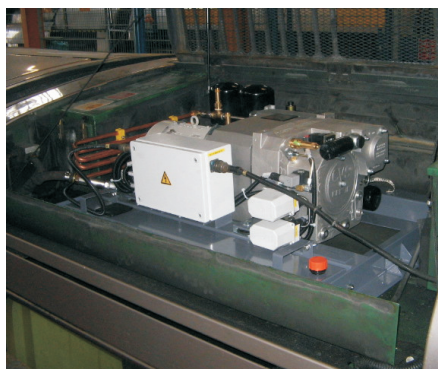
Figure 18: Example for roof mounting without cover
