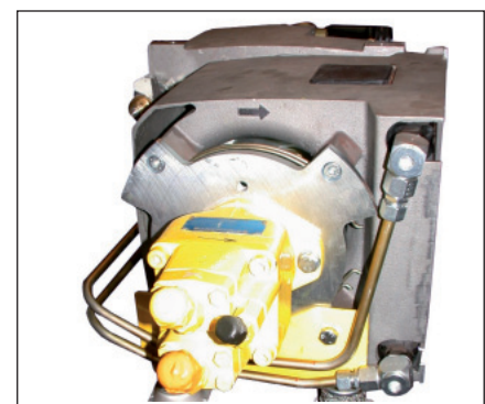
Figure 6: Drive with hydraulic motor
